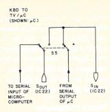
Fig. 4. Switch S5 wiring.
